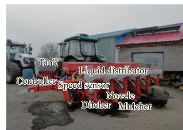
Figure 6 Soybean seeder equipped with control system
