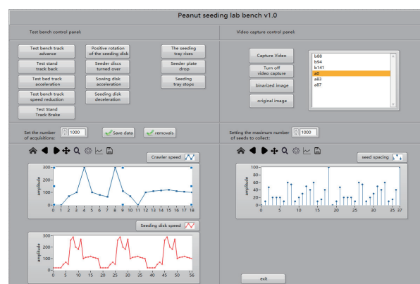
Figure 15 Upper computer interface of test bench
