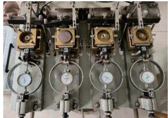
Figure 3 Soil direct shear test
