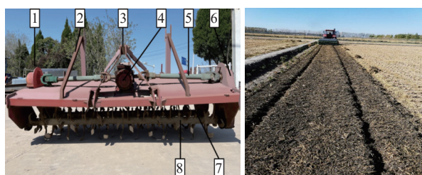
1. Siderear transmission gearbox 2. frame 3. Three-point suspension device 4. Intermediate transmission gear box 5. Transmission shaft 6. side front transmission gearbox 7. backward rotary blade group 8. forward rotary blade group
