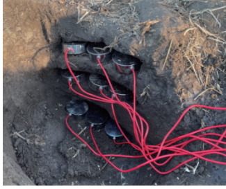
b. Soil stress and pressure acquisition equipment
