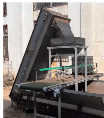
Figure 13 Test prototype of filling device
