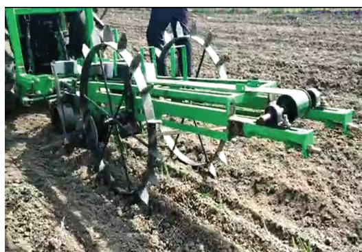
b. Field working of developed onion transplanter view
