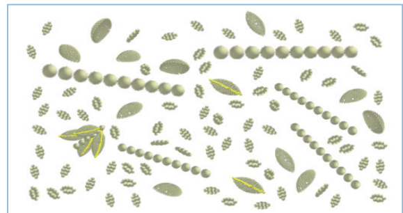
Figure 14 Calculation of non-threshing rate by simulation experiments
