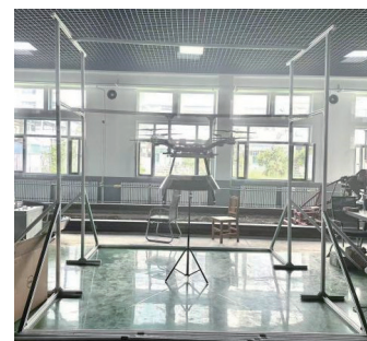
Figure 8 Plant protection drone test bed structure diagram
