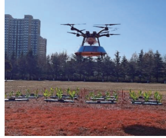
Figure 11 Field spraying test under soybean-maize complex planting pattern
