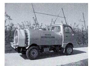
b. 3WZ-700 self-propelled orchard airflow directional sprayer [53]
