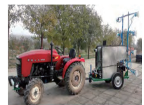
d. Orchard automatic profiling sprayer [56]
