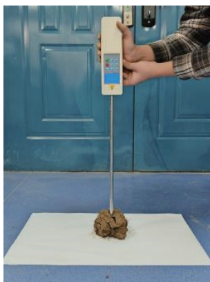
Figure 4 Soil block firmness detection test
