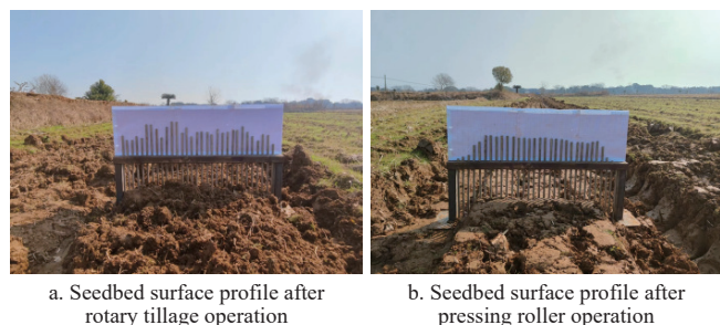
Figure 13 Field experiment of pressing roller operation
