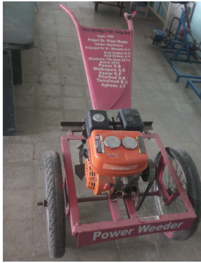
Figure 5 Developed two-row tyned weeder
