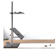
a. Device for determining the coefficient of recovery of peanut pods-65Mn steel plate collision
