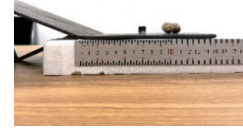
a. Rolling friction coefficient determination test device
