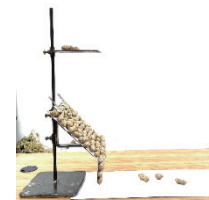
c. Device for determining the coefficient of recovery of peanut pod-pod collisions
