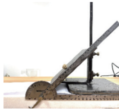
a. Test device for determining the coefficient of static friction
