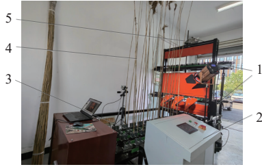
1. Conveying device; 2. Test control platform; 3. Feeding device; 4. Reed stalks; 5. Three asynchronous motors
