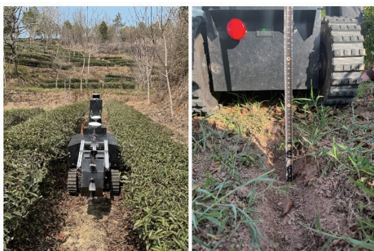
Figure 10 Experimental setup of the electric rotary tiller in field operation
