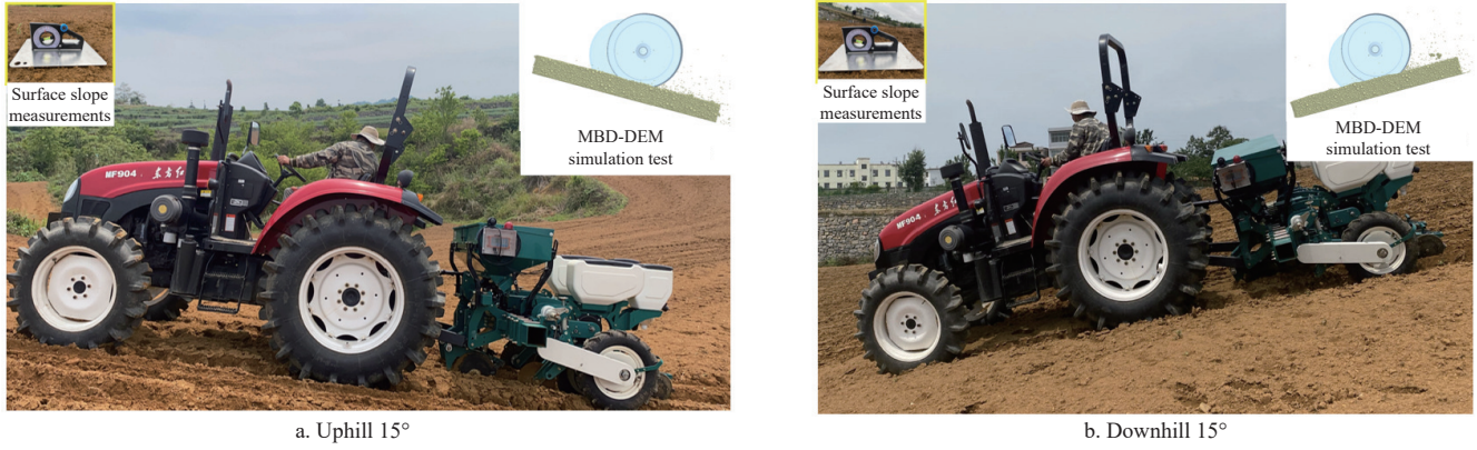
Figure 9 Simulation and field validation tests of furrow opening operation
