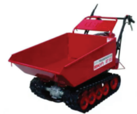
b. IBT-500RDH portable crawler transporter
