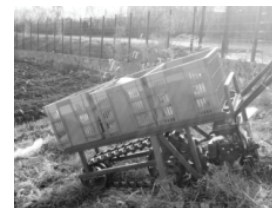
a. Small hand-guided single-crawler transport vehicle
