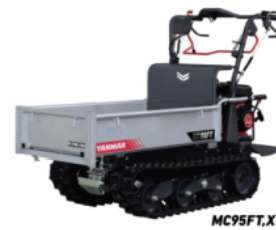
c. Yanmar MC95FT-X crawler transporter
