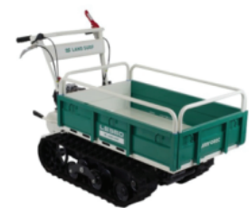
d. Orix LS-360 portable crawler transporter
