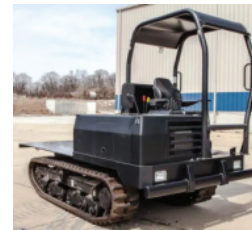
a. EX60 multi-functional crawler transporter
