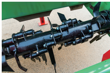
Figure 6 General assembly of potato vines removal cutter [15]
