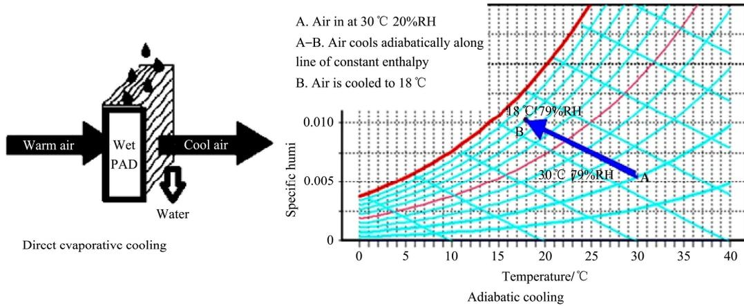
Figure 1 Schematic of direct evaporative cooling (Source: www.ecocooling.co.uk/psychr.html)
