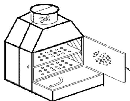
Figure 10 Evaporative cooler
