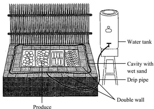
Figure 7 Evaporative cooler made from bricks
