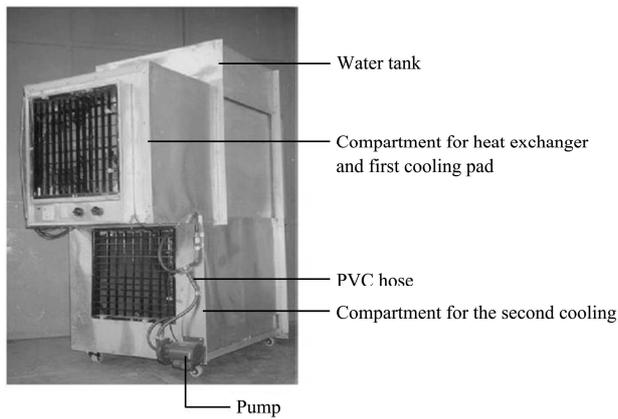
Figure 11 Indirect active evaporative cooler
