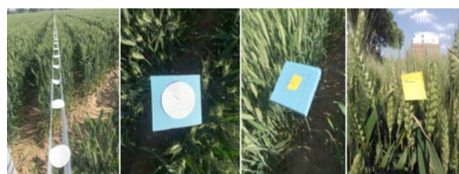
a. Crosswise filters b. Longitudinal filter c. Horizontal WSP d. Vertical WSP
